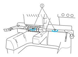
① Use the thumb screws included with the machine (thumb screws removed in step ① on page 171).
